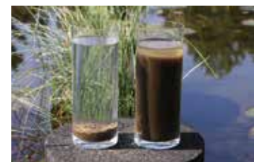
SVI 5 comparison of aerobic granular sludge (left) and conventional activated sludge (right)
