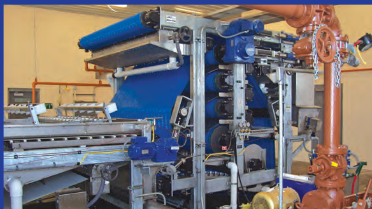
Dual Purpose 2 meter model 3DP , Licking County, OH Operates as a Gravity Belt Thickener or Belt Press.
