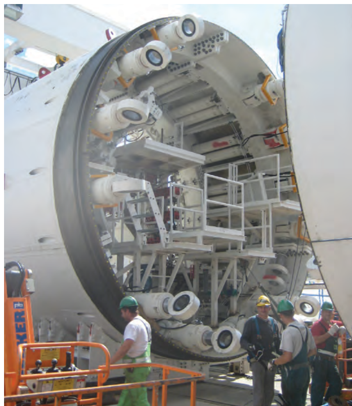
TBM (tunnel boring machine) being manufactured at the Herrenknecht plant in Germany. (Kenny Construction)
