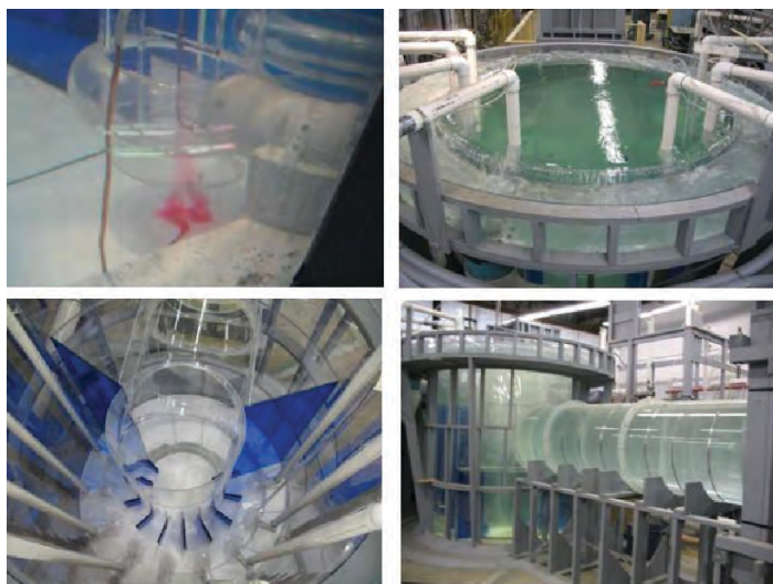
This is the physical model built to evaluate the pumping system hydraulics for the OARS tunnel. (Northwest Hydraulic Consultants)
