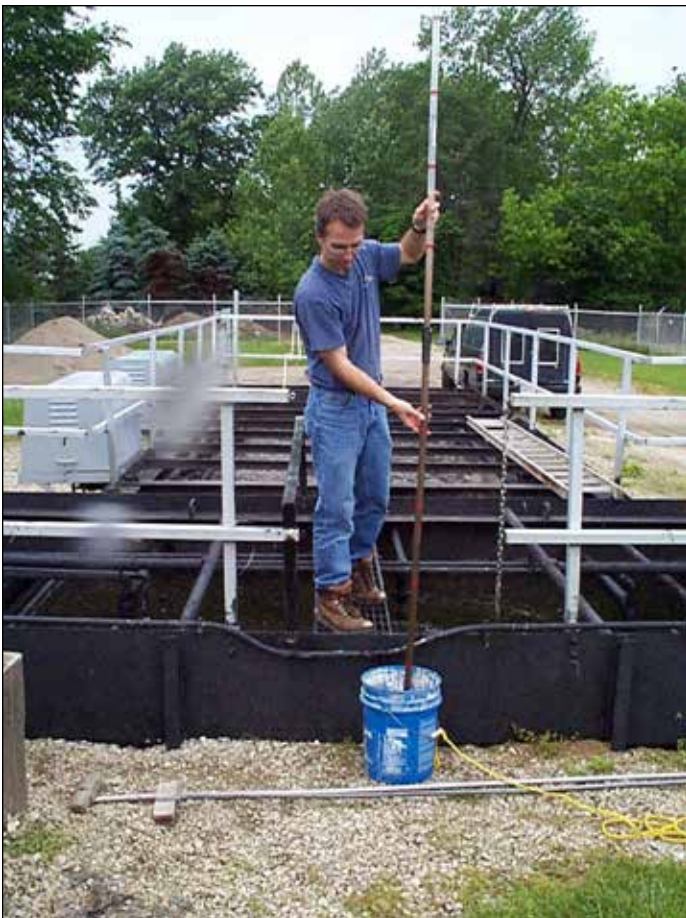
Figure 3: Emptying a Clarifier Core Sample into a Bucket
