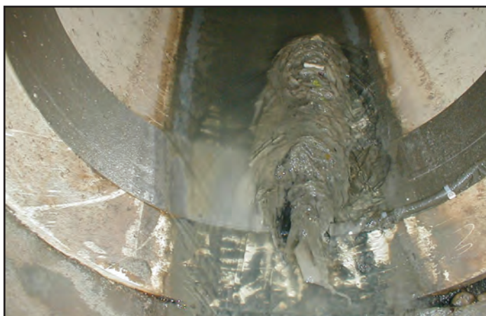
Figure 3: Debris run straight into the face of a normal probe at low flow
