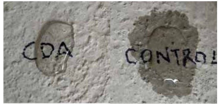
Figure 4: Concrete produced with a permeability-reducing admixture – hydrostatic (also referred to as a concrete densifying admixture, hence “CDA”), left, and concrete produced without a permeability-reducing admixture (also referred to as the reference or “control” concrete), right. (Concrete Sealants, Inc. file photos)
