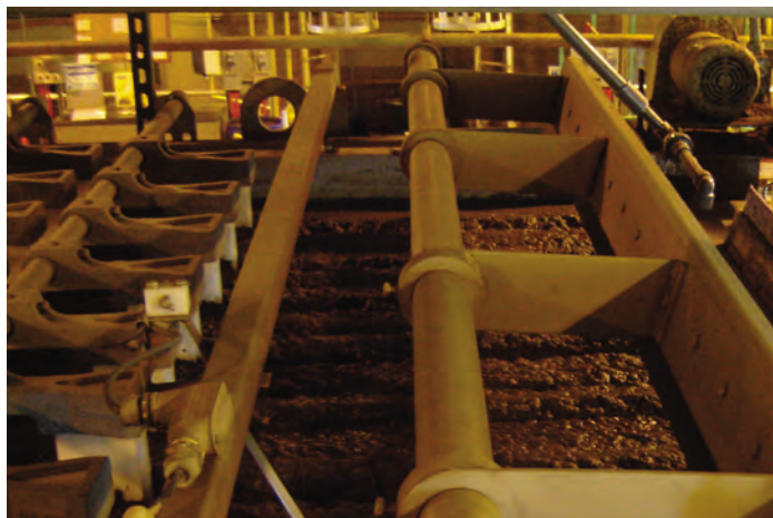
Belt filter press gravity zone
