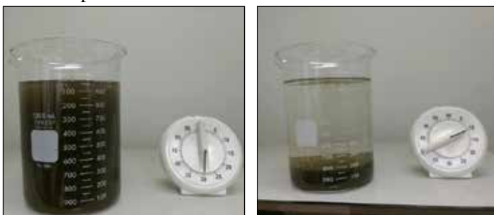
Settleometer Tests at Time 0 and 10 Minutes Compliments of Andy Krispinsky, City of Aurora Ohio
