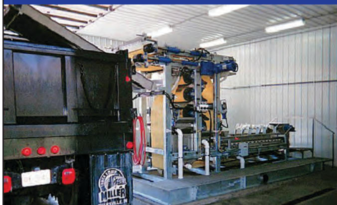
0.5 meter BDP Heavy duty machine designed for small plants. Millersport, Ohio
