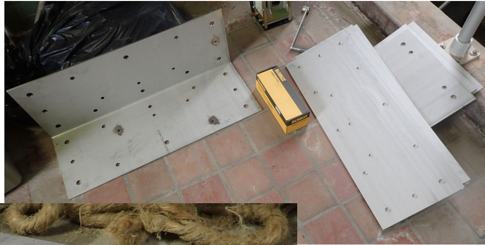
Fabricated Bent and Flat \frac{1}{4} ' Thick SS Plates
