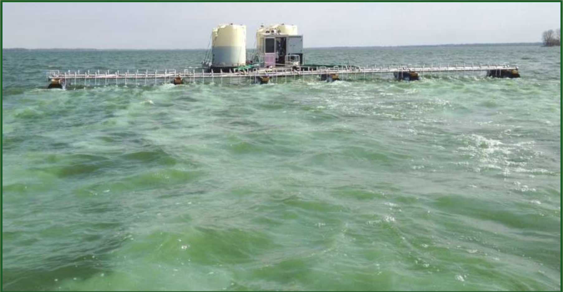
HAB Chemical Application Barge in Operation
