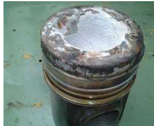
Siloxane damage to upper cylinder area and piston
