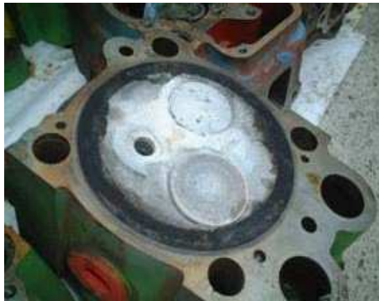
Siloxane damage to upper cylinder area and piston
