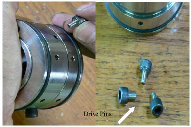
• Separate the cartridge halves and remove seal faces.
