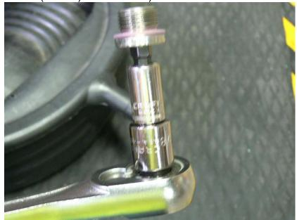
13. Remove the pump volute by removing six (6) hex head bolts and lock washers (19 mm socket/wrench) and, using the hoist for the lift, pull the motor with the impeller attached out of the volute. If the volute sticks to the motor housing, use rubber mallet on the volute to release unit (6" or less above the mat).
