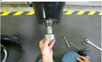
Remove the mobile portion of the mechanical seal by hand or with the cotter pin puller.
