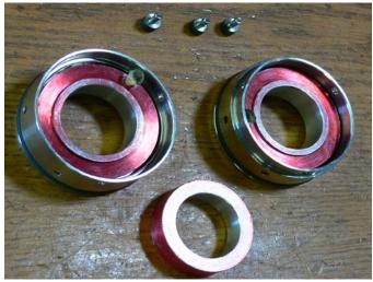
• Press cartridge halves together, insert the three (3) drive pins.
