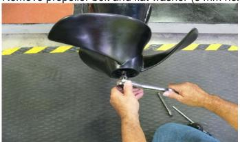
Slide propeller off the splined shaft.
