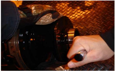
Remove impeller bolt, special lock washers and bushing (17 mm socket and 6" extension).
