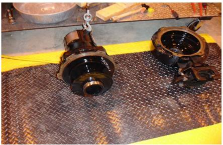
16. Remove the impeller.
