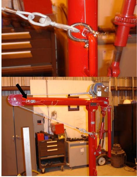
9. Reaching from the side of the platform attach the hoist hook to the clevis on the mixer.
