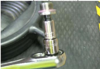
15. Drain oil from gearbox (when facing propeller, left side, back plug).
