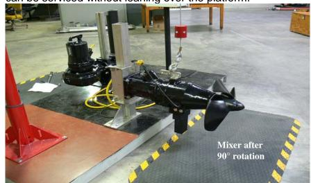
11. Place oil drain pan on floor under the pre-chamber and gearbox drain plugs.
