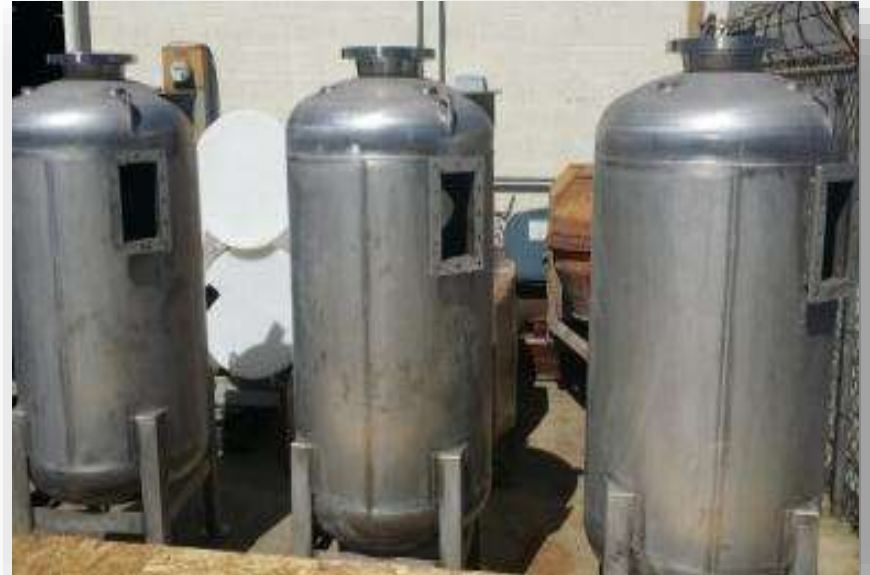
Pilot Digesters Awaiting Delivery to Encina
