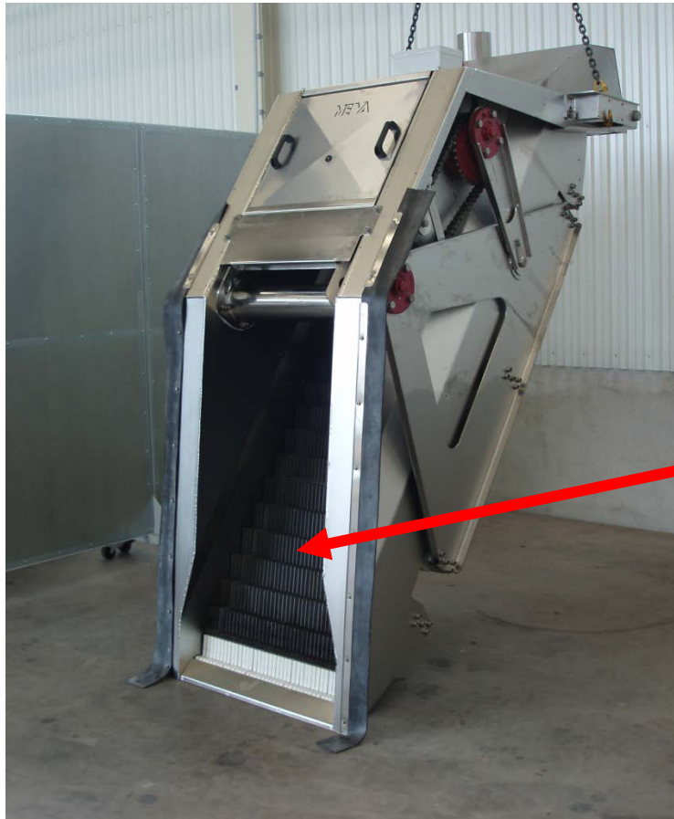
“Step” shaped bar forms screening surface
