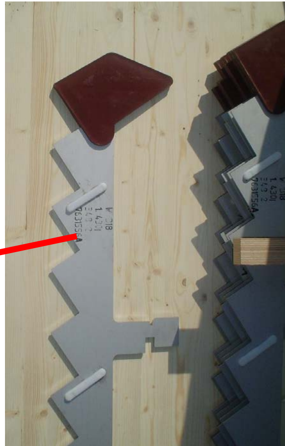
“Step” shaped bar forms screening surface
