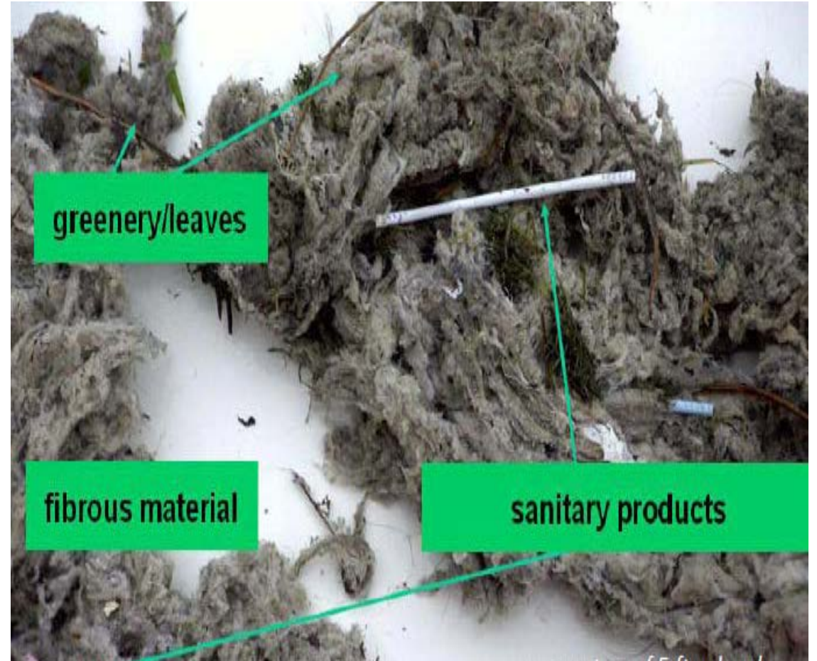
Material from a clogged MBR system
