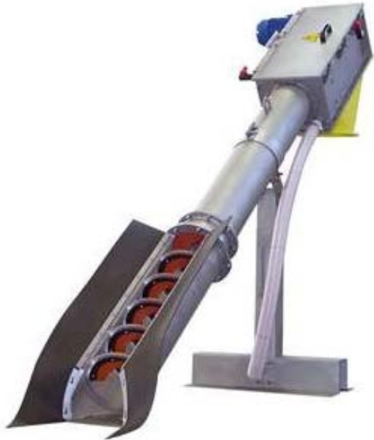
Rotating Screw - with brushes and Perforated Plate Screen
