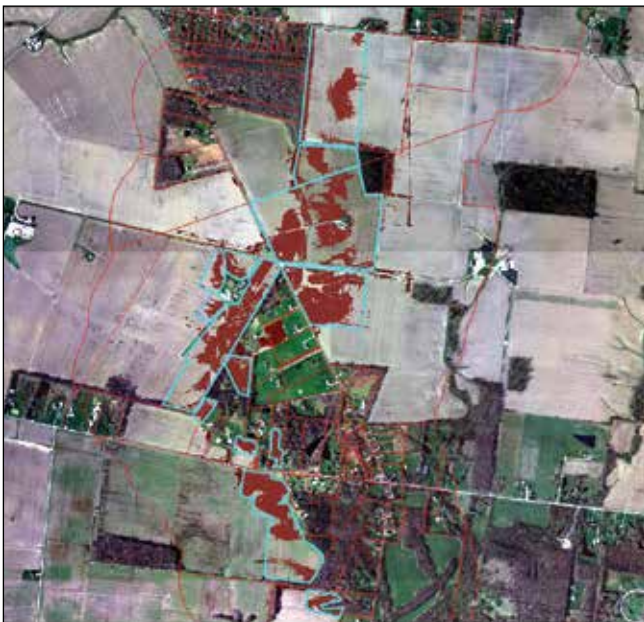
SWAT model simulation shows areas of high sediment yields. The highlighted fields were targeted for cover crops.
