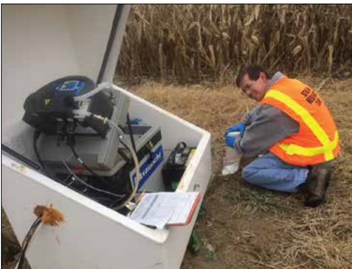
Clermont SWCD staff collect samples from one of four autosamplers at the capture BMP.
