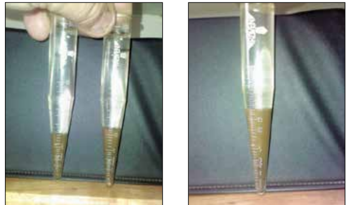
Figure 2 & 3: Process control centrifuge tubes showing high solids in aeration tanks with spin values of 10, 15 and 20. Typical aeration tank spins are 2-4.
