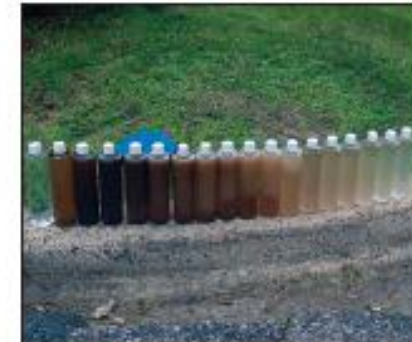
ICE PIGGING process samples from start to finish
