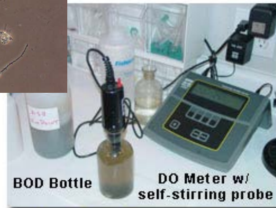
Dissolved Oxygen Uptake (DOUR) Test
