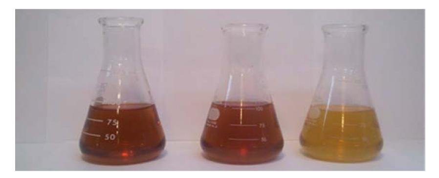
Color change of biologically treated leachate with various oxidants (left to right: before oxidation, with ozone only, and with ozone and hydrogen peroxide)
